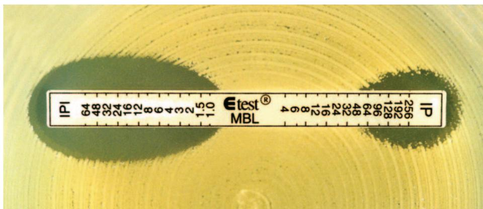
FIG. 4. Etest MBL strip (reprinted with permission from AB BIODISK, Solna, Sweden) and an *Acinetobacter* sp. expressing a VIM-2 MBL. The intersection of the ellipses at the strip is read from two halves, i.e., at the section with imipenem alone (IP) and imipenem plus EDTA (IPI). A reduction in the MIC of imipenem of  $\geq 3$  dilutions in the presence of EDTA is interpreted as a positive test.
